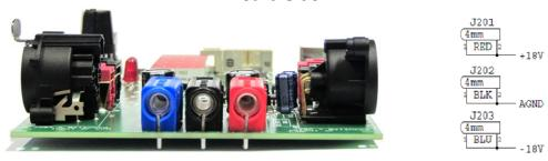
The side of the board has three connectors for analogue power. The red is +V, blue -V and black analogue ground. Maximum voltages are in the recommended operating conditions section.
