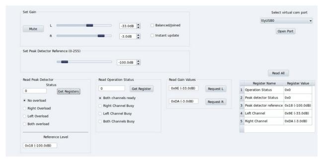
The GUI program runs on Linux, Windows and Mac OS X. All functions of the MAS6116 can be changed from and read by the program. There is only one screen and all functions can be changed from this screen.
