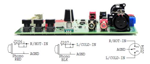
The front of the board has three audio connectors. The right hand XLR socket is for balanced audio in; the two phono sockets are for single ended audio in, with red the right channel and black the left channel.
