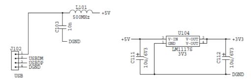
The digital section is powered from the USB connector. It can be powered from a standalone power supply with a USB plug as long as it complies with the specifications given in the section "Recommended operating conditions".
